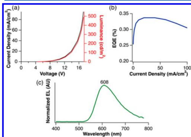
Figure 8. ITO/MoOx/NPB/**2**/LiF/Al device. (a) Current density and luminance characteristics. (b) EQE data with a maximum of 0.34%. (c) EL spectrum of the device with  $\lambda_{\text{max}} = 608$  nm.
